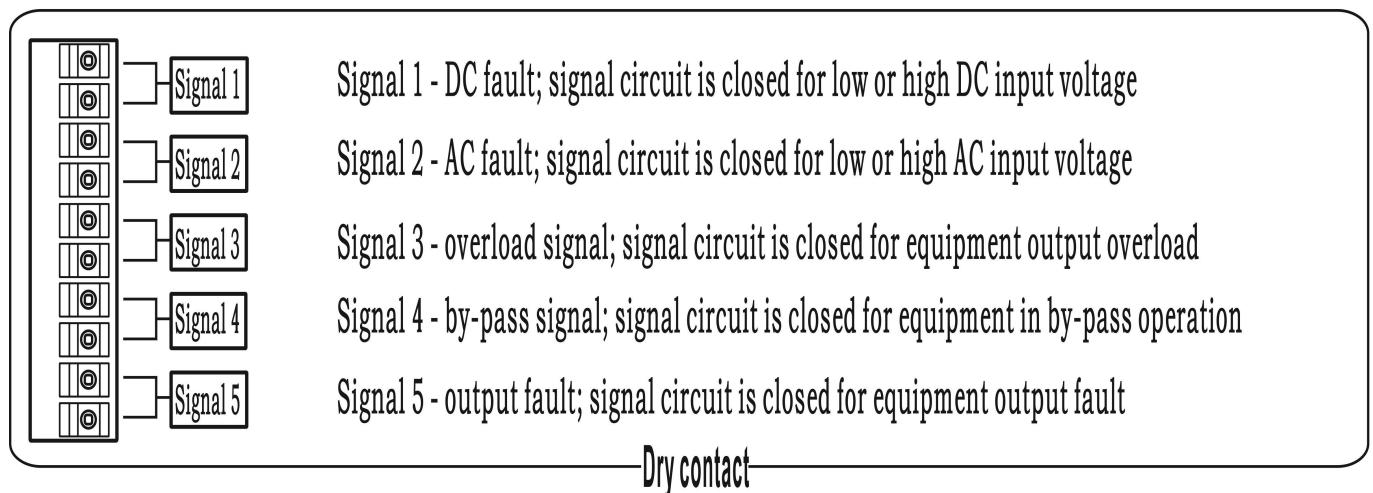
**Note: the contact capacity of each group of the dry contacts shall not exceed 60 V 0.5A.**
